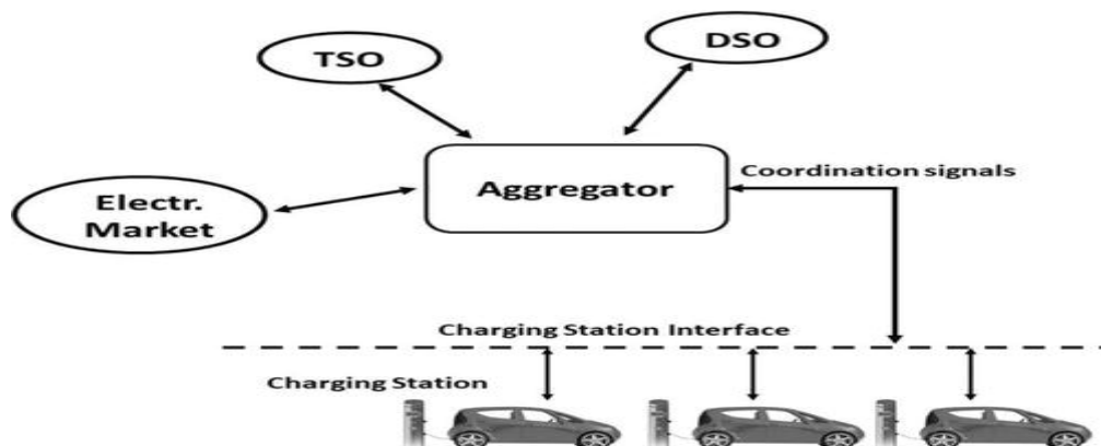
Figure 1: Simplified EV coordination framework: transmission system operator (TSO), distribution system operator (DSO), electric market, and charging stations for EVs.
