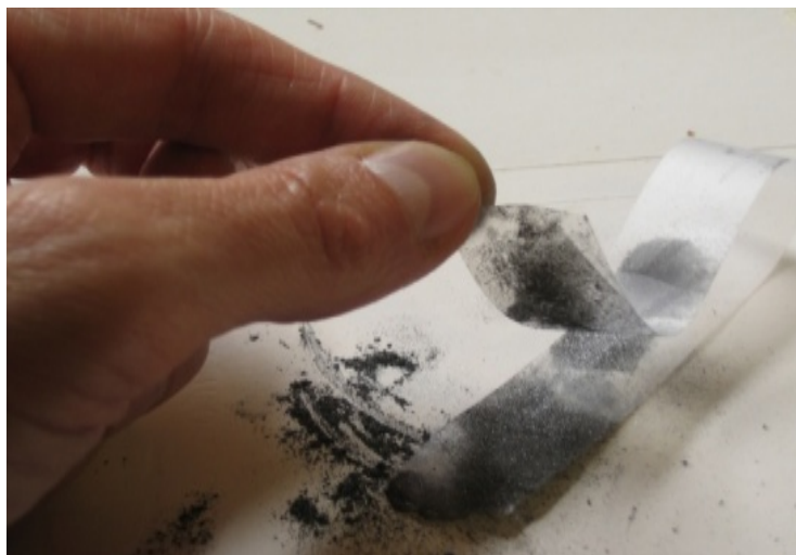
Fig 2: Making Graphene using sticky tape
