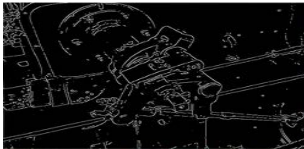
Figure6: Image after applying Canny edge detector
