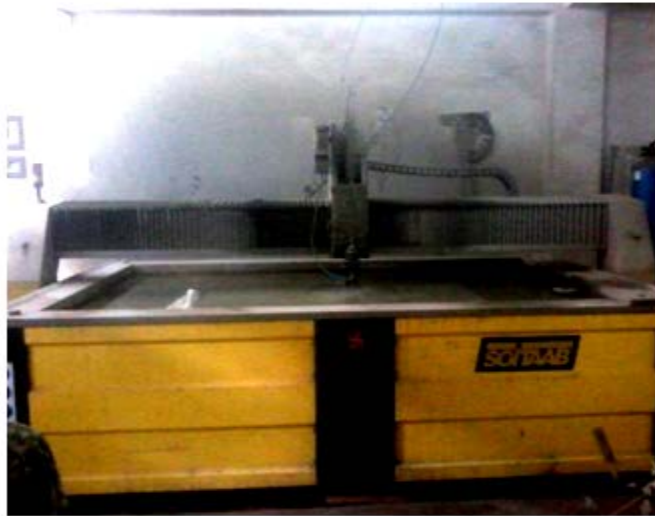
Figure 1: Abrasive water jet machine & components
