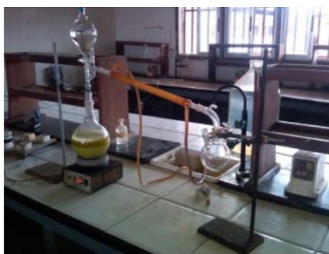
Figure 2: laboratory set up for steam distillation of citrus peel.
